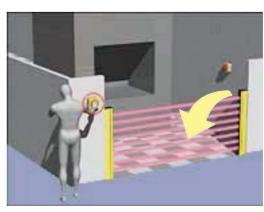
The worker gets out from the zone and presses the B button. He must do it in scheduled time to reset the machine.
