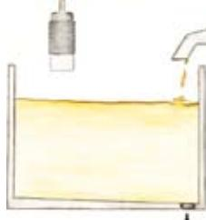
Overflow protection of casts, for example for plastic lenses for glasses with capacitive sensors of the KXS-Extreme series.
