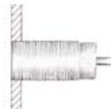
The **non-flush** mountable sensors are designed for applications, in which the medium to be monitored comes in direct contact with the sensor. In such level monitoring systems, the sensor head is completely immersed in the powder, granulate or liquid.
