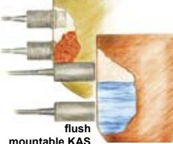
Detection of the content of a cardboard package e.g. tins with capacitive sensors (KAS)
