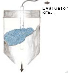
Level control of different media with TRUE- or PER Level rod probes with connection head (KFX)
