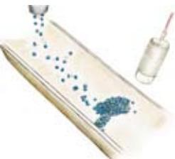
The capacitive filling level measuring systems (KFS/KFA; KFX) operate according to the three-electrode principle. Here the container or an additional electrode serves as a counter-electrode to the probe electrodes. For this reason it is essential with this system that the container is of a conductive material or a „substitute electrode“ is fixed to the container wall, e.g. copper foil.
